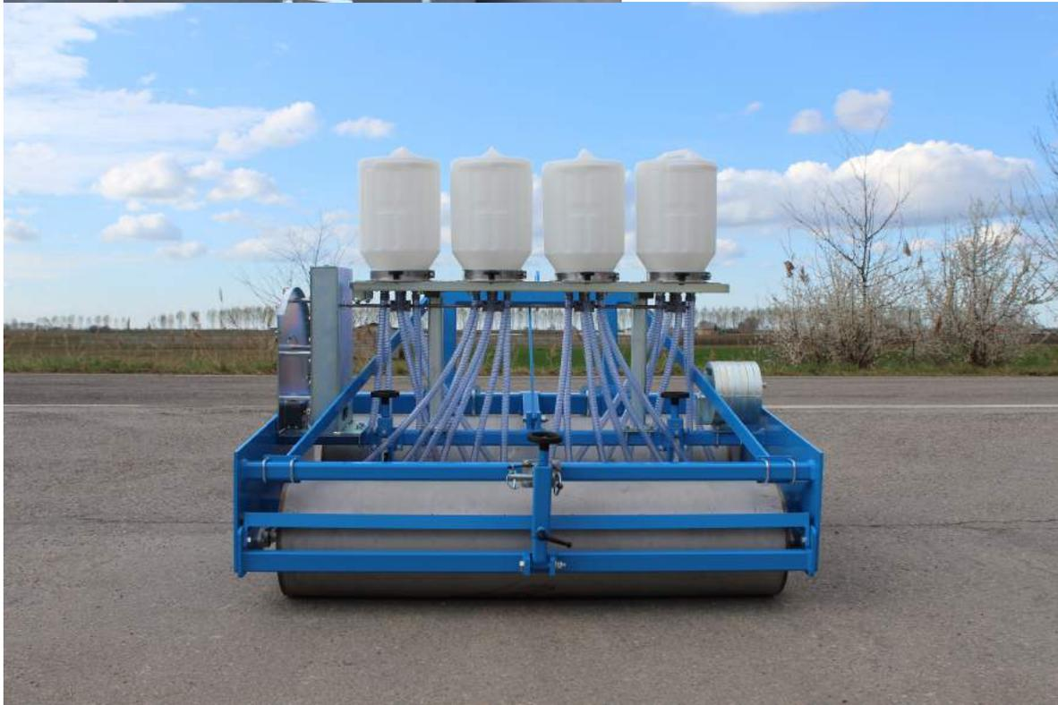
The *mechanical system* has no maintenance problems and does not require qualified personnel, because it is sufficient to position the arrow at the desired number to decide the quantity of seed that falls. It is ideal for large surfaces in the open field.
