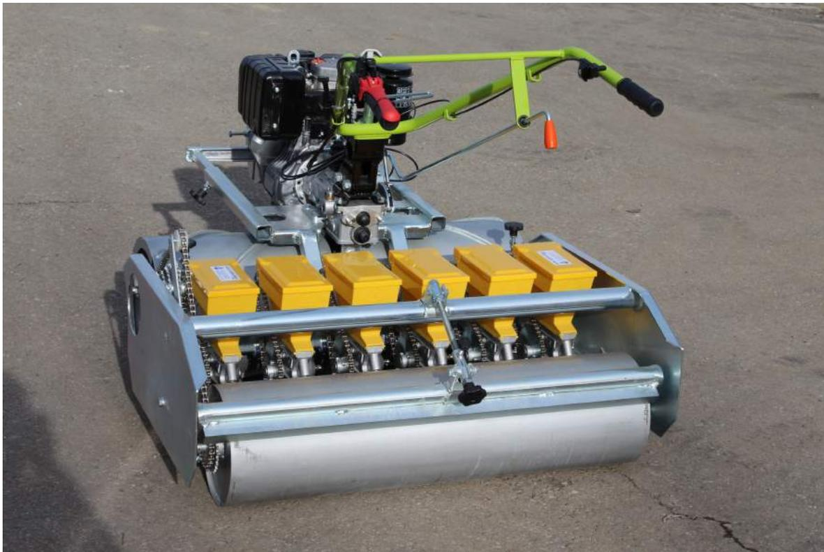
The **SP 94** model was created to perform first rolling, sowing and second rolling to cover the seed in a single operation, in order to considerably reduce processing times.
