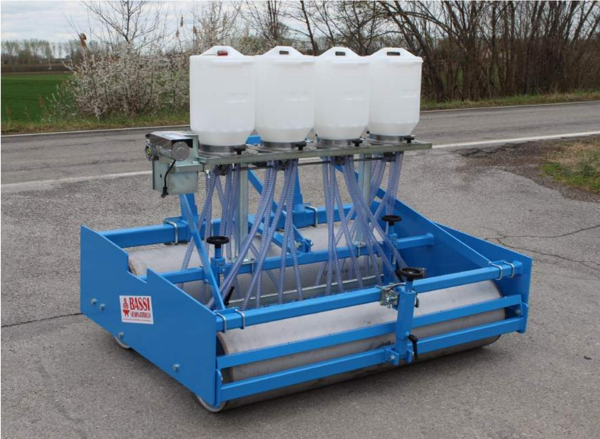
In the *electronic system*, the movement of the sponge is transmitted by a 12 V electric motor: by varying the speed of this motor with a convenient control, you can adjust the quantity of seed coming out. It is possible to sow from 1 to 1000 kg / Ha. This model is more precise as regards calibration, it allows you to program the dosage even if you change the type of seed. However, more attention is needed in programming the machine and specialized personnel is required.
