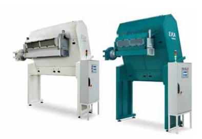
EXA is a forefront system designed to grant comprehensive and accurate detection of contamination in Spinning and in Nonwovens Industries. EXA implements robust technologies to face the critical conditions of blow room lines.
