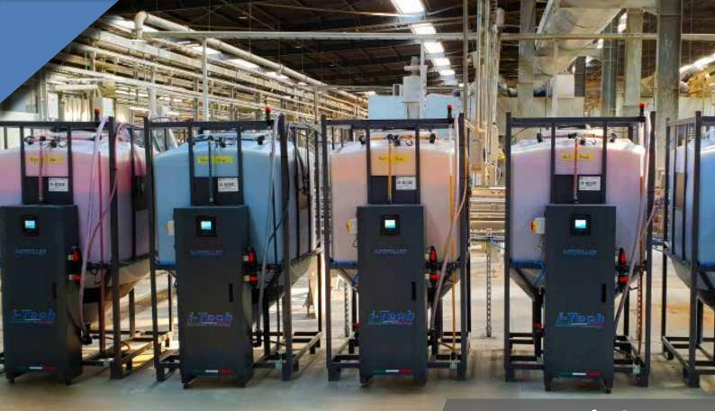
I-NKFILLER® is the innovative I-Tech transfer system for an automatic refill of digital printers' reservoirs from storage tanks entirely conceived and created by I-TECH.
